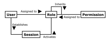
Fig. 1: UML Class Diagram: Hierarchical RBAC Model
